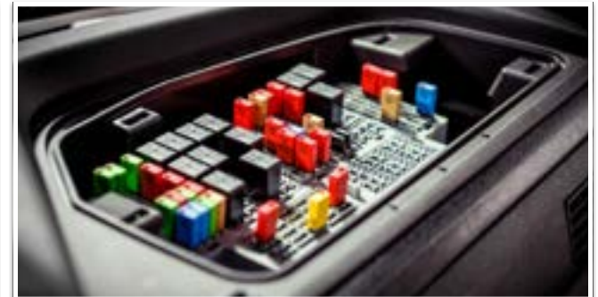
In-cab electrical panel is protected from the elements and conveniently located under spill-resistant dash panel
