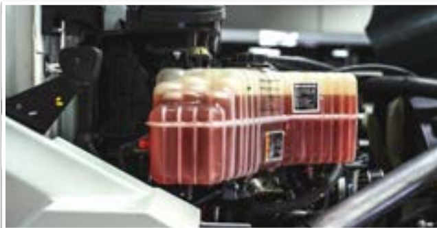
Key fluid reservoirs are translucent for quick inspection and many of the caps are tethered, saving time and frustration from dropped or lost caps
