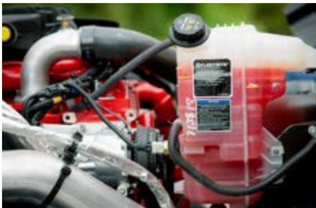
Tethered caps on most fluid containers prevent dropped or lost caps while refreshing fluids.
